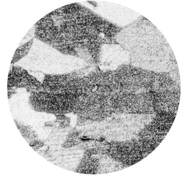
Figure 2: Rolled lead, magnification x 30 Etchant: Voces Reagent
